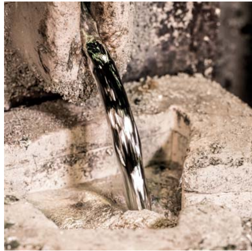
Smelting of the zinc with alloying elements (copper and titanium).
