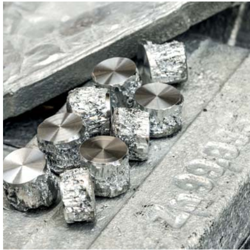
Zinc crystals from zinc compliant with European Standard EN 1179.
